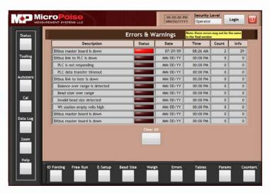
The Errors & Warnings screen is a great tool for trouble shooting the machine. This feature helps operators to identify potential system problems in order to maximize uptime.
