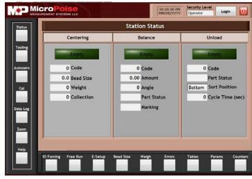
Input output forcing allows for digital diagnostics while observing communications between the computer and the PLC.
