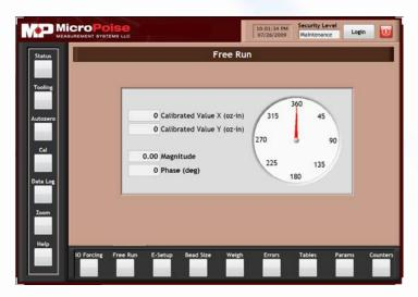
The Free Run screen offers users the ability to perform maintenance and system diagnostics. Raw and scaled voltages can be observed.
